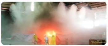
A Water Mist System is a type of fire suppression system that uses a fine mist of water droplets to extinguish fires. Water mist systems are commonly used in areas where traditional water-based sprinkler systems are not effective or may cause more damage, such as in sensitive electronic equipment rooms, museums, libraries, or historical buildings.
